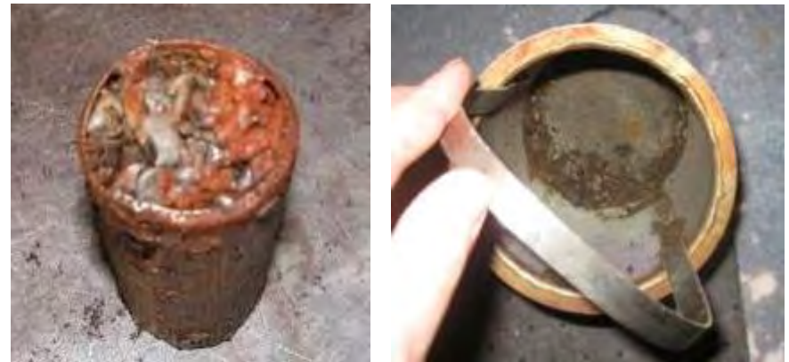
Strainer basket from untreated bearing cooling water supply (left) and treated with HOD UV (right)
