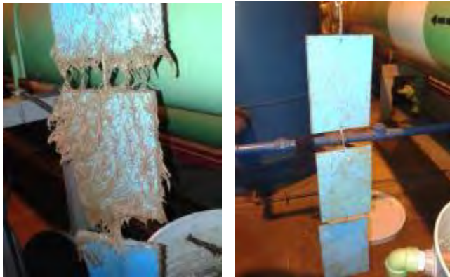
Sampling plate from untreated bio-box (left) and treated with HOD UV (right)
